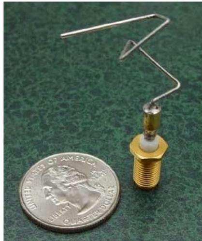
FIGURE 4: The 2006 NASA [ST5](#) spacecraft antenna, a topology discovered by an evolutionary algorithm to have the best radiation pattern.
